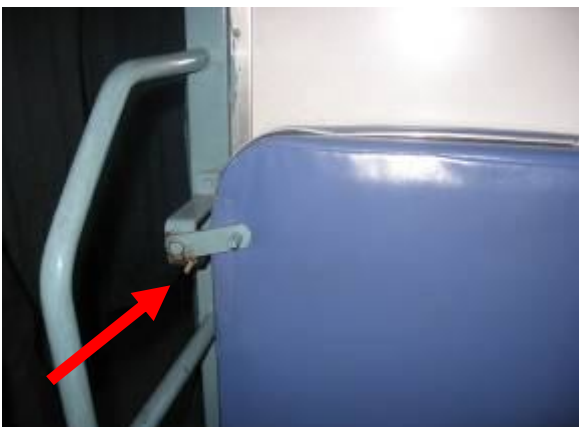
Modified latch for Berth cum back rest
