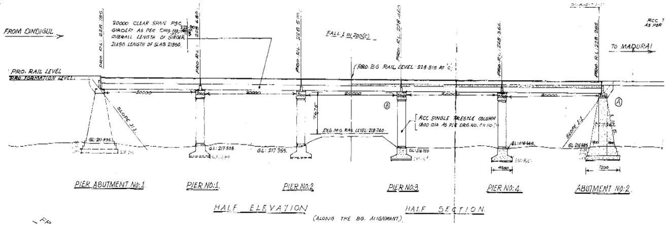
Figure 2 Elevation of PSC Girder Bridge 1377A
