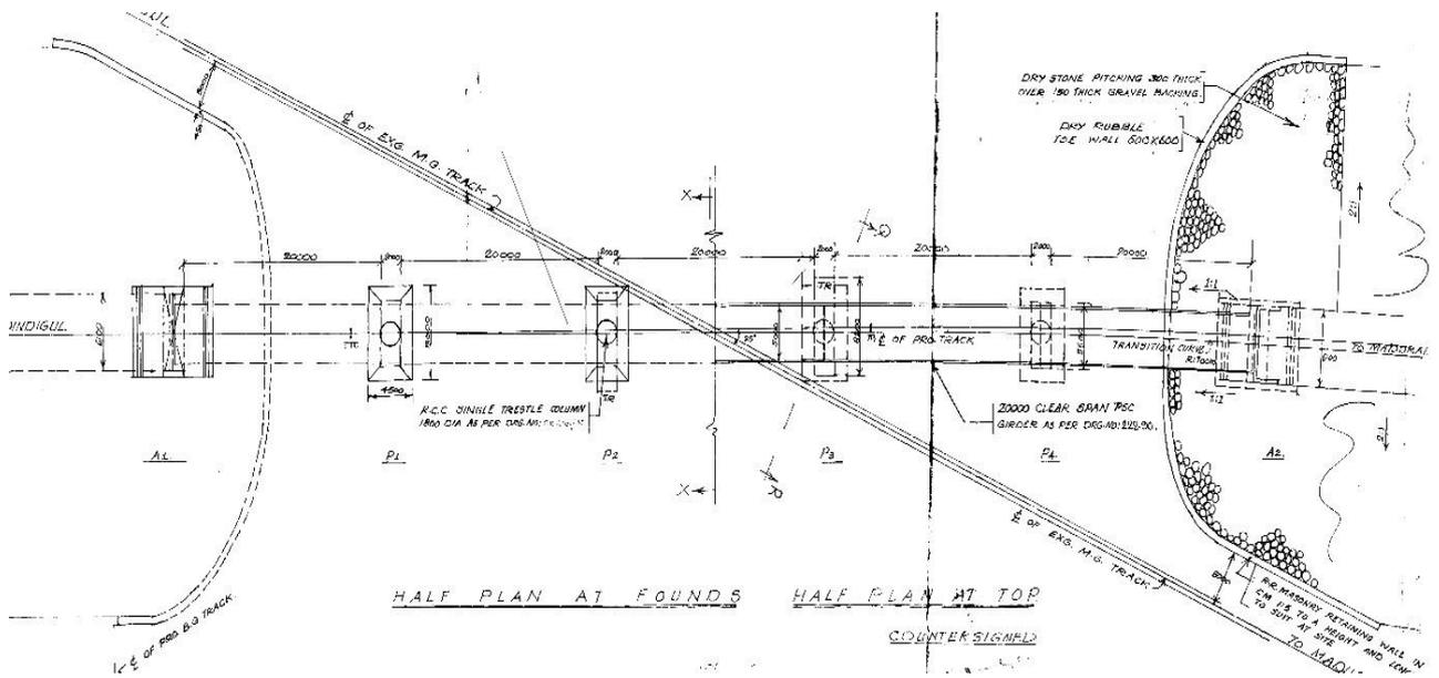
Figure 3 Top view plan of PSC Girder Bridge 1377A
