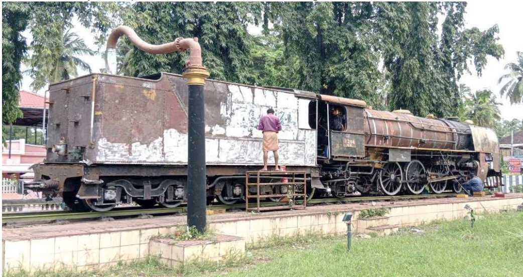
d. Application of Putty and primer for surface finishing
