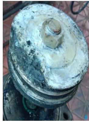
Piston Disc (Water side) found decayed
